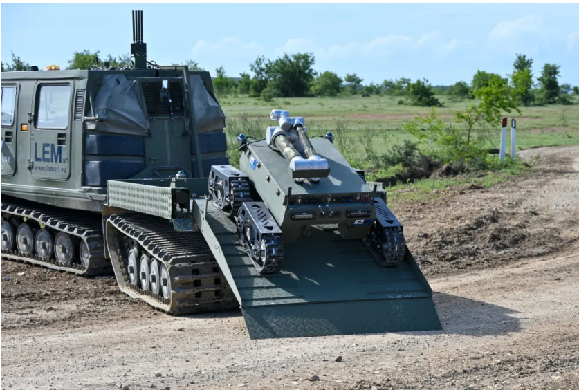
Unloading phase of the LEM Small Tracked UGV ArmScout1 from the rear ramp of the BV206. Source: Italian Army.
