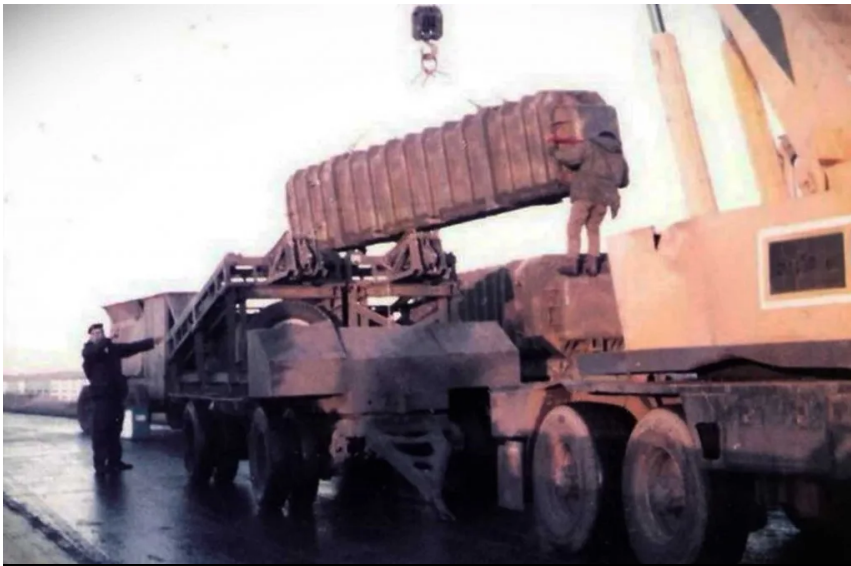
The Exocet battery installed in the improvised cart at Puerto Belgramo, in mainland Argentina, during May 1982.
