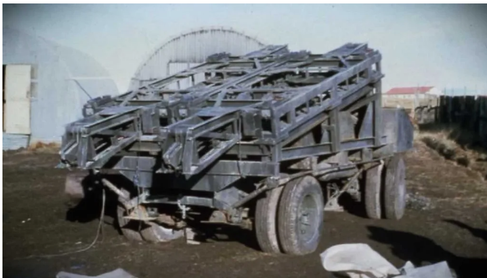
The cart that transported the Exocet to be launched from land. During maneuvers, it was transported by an agricultural tractor.
