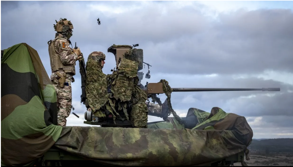
The 20 mm PROTEUS cannon targets an enemy drone. The automatic weapon has been specifically adapted for anti-drone defense. Photo: caporal-chef de 1re classe Yann Dupuy.
